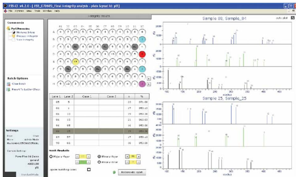
Figure 2. Contamination. The FSS-i3™ Expert Systems Software has a feature called i-integrity. i-integrity evaluates all samples in a batch for well-to-well contamination. Three different match criteria compare peaks: major-to-major; major-to-minor; and minor-to-minor. The three different match components can be used to evaluate splash over, general contamination from an analyst and duplicate samples.
