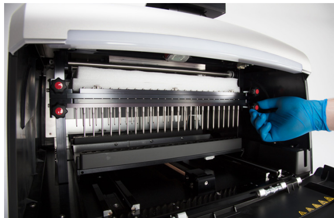
Figure 63. Placement of plastic stoppers. Move the magnet and plunger bars up, and secure the four shipping screws on both sides of the magnet and plunger bars.
