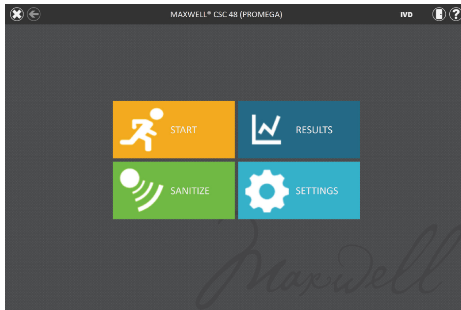
Figure 57. 'Home' screen. Selecting the Sanitize button begins the process for UV treatment of the Maxwell® CSC 48 Instrument.
