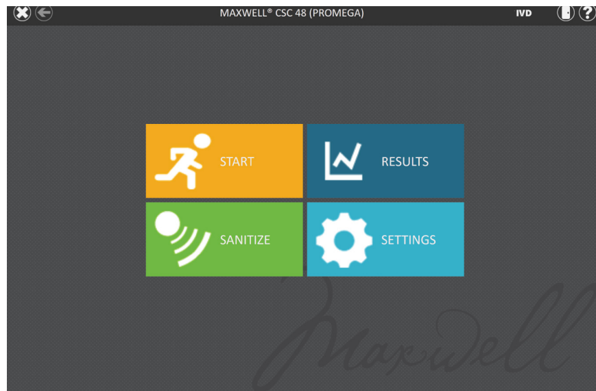
Figure 54. Maxwell® CSC 48 'Home' screen. Selecting Results opens the Maxwell® CSC 48 'Results' screen from which extraction reports from all method runs can be viewed.
