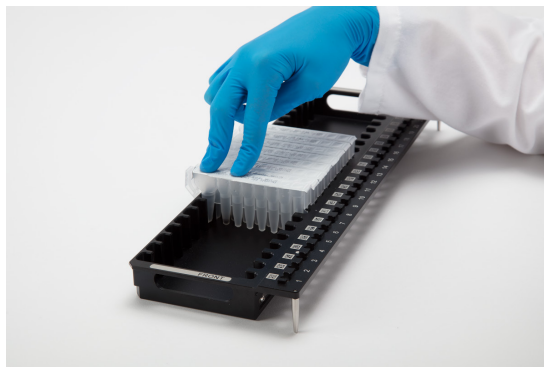
Figure 40. Placing the cartridges in the Deck Tray and pressing firmly to snap them in place.
